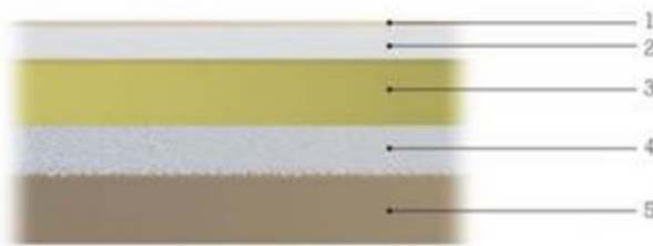
Figure 2: A ground slab normally consists of several layers and a theoretical structure is: 1. Floor covering, 2. Concrete slab, 3. Heat insulation, 4. Capillary layer (single, gravel) and 5. Ground
